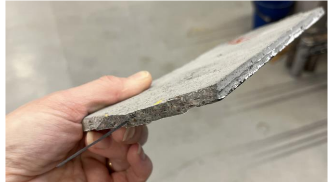
Concrete with embedded carbon fibre textile. Photographer: Chalmers | Catharina Björk
