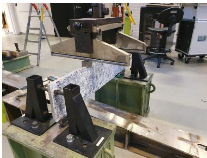
Test set-up where textile-reinforced concrete is loaded in the construction lab at Chalmers. Photographer: Chalmers | Catharina Björk
