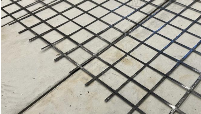
Carbon fiber textile reinforcement mesh. Photographer: Chalmers | Mia Halleröd Palmgren
