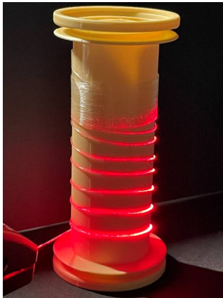
Spun light: These polymer fibers conduct light and are produced using a new microfluidic wet spinning process. Image: Empa
