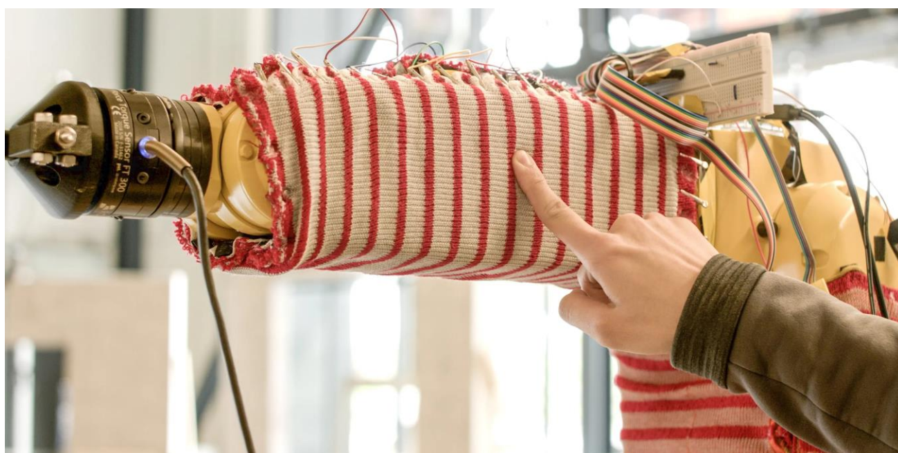
RobotSweater, developed by a research team in the Robotics Institute and shown here on a robotic arm, is a machine-knitted textile "skin" that can sense contact and pressure.
