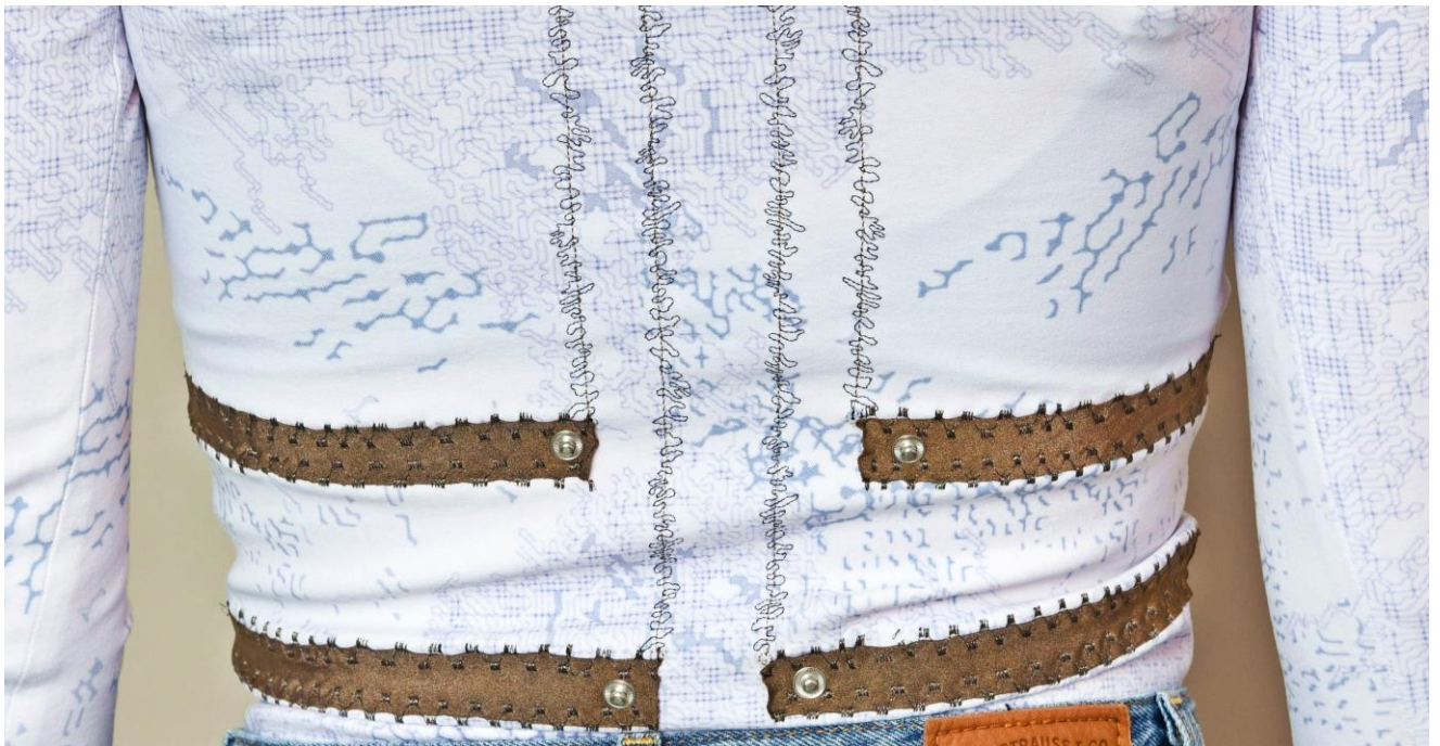
A shirt that monitors breathing: Designer Laura Deschl developed the monitoring system to wear together with Empa. Image: Empa
