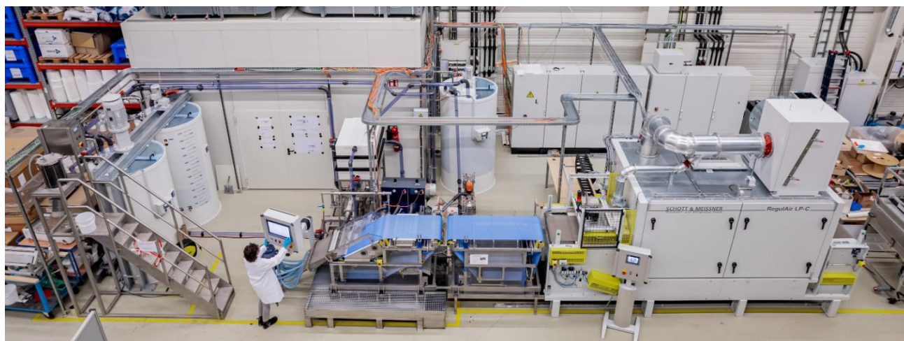
Nassvlies Pilotanlage © A3/Christian Strohmayer
